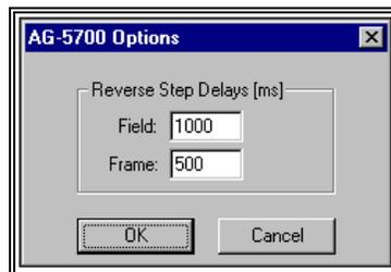
Due to the mechanical nature of the 5700 VCR, it is difficult to reverse one field at a time. The VCR must receive a Frame Reverse command, wait for the counter to change, delay while the VCR settles down and then issue a single Field Advance command.
