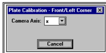
The user must first specify the location of the video camera in relation to the force plate. This axis is relative to the force platform coordinate system and represents the axis projecting from the center of the platform to the camera. Available selections are X, -X, Y and -Y. Then digitize the four corners of the plate as instructed. Digitizing begins with the Front-Left corner of the plate and proceeds with Rear-Left, Rear-Right, and Front-Right corners.
