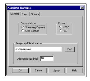
5. Select **Streaming Capture**, specify the video **Format**, set **the Temporary File Allocation** and **Allocation Size** for the AVI file.
