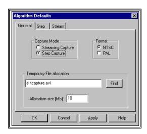
5. Select **Step Capture**, specify the video **Format**, set **the Temporary File Allocation** and **Allocation Size** for the AVI file.
