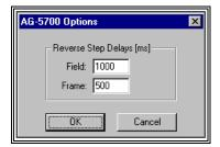
Due to the mechanical nature of the 5700 VCR, it is difficult to reverse one field at a time. The VCR must receive a Frame Reverse command, wait for the counter to change, delay while the VCR settles down and then issue a single Field Advance command.
